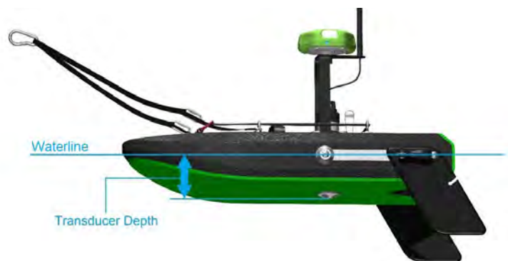
Figure 1. Transducer depth shown with the SonTek-RS5 on a HydroBoard II - Micro.
