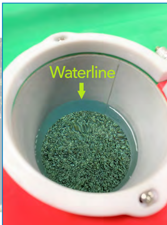
Figure 11. Waterline inside the ADCP hole.
