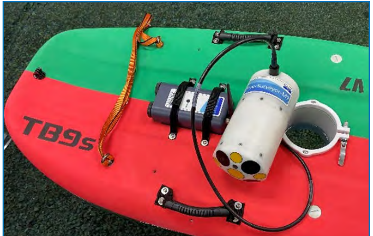
Figure 10. ADCP setup with M9 on Torrent Board.
