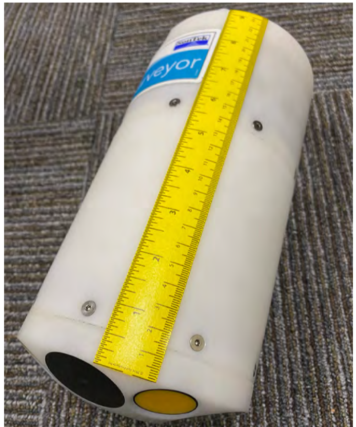
Figure 14. SonTek-M9 with graduated sticker ruler.
